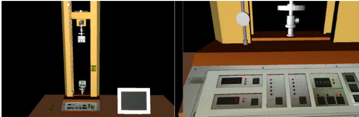
Figure 4: Overall view and the instrument panel of the Tensile Testing VR apparatus
