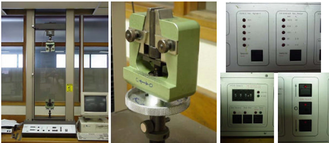
Figure 2: Hounsfield Tensile Testing Machine and some details
